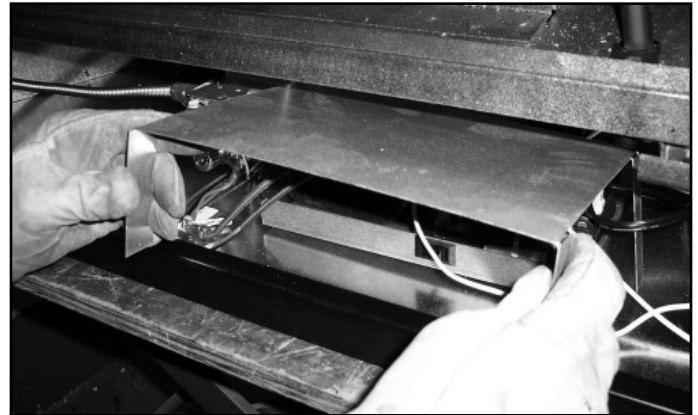
Figure 12.6 Placing Remote Cover Plate
